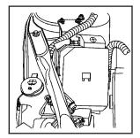
To uncover the remote positive (+) terminal, remove the fuse block cover. You should always use the remote positive (+) terminal instead of the positive (+) terminal on the battery.
